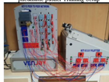
Peer to Peer network and X-Y Plotter
