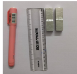
Impact test samples prepared by CNC machine
