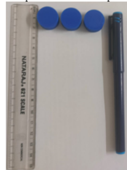
3D printed compression & hardness test samples
