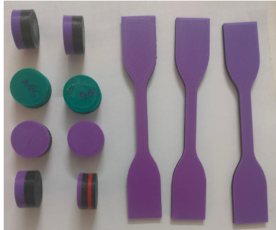
Samples Prepared through 3D printer
