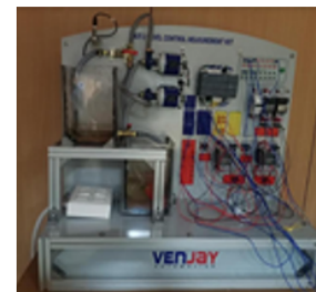
Level Control Measurement Training Setup with PLC
