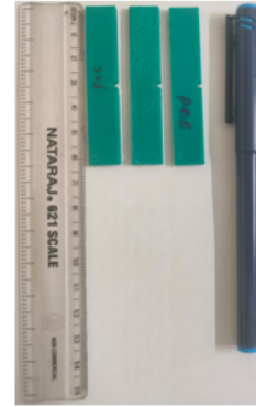
3D printed impact test samples
