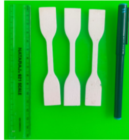
3D printed tensile test samples
