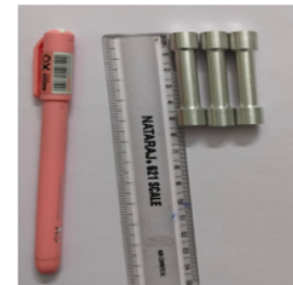
Tensile test samples prepared by CNC machine
